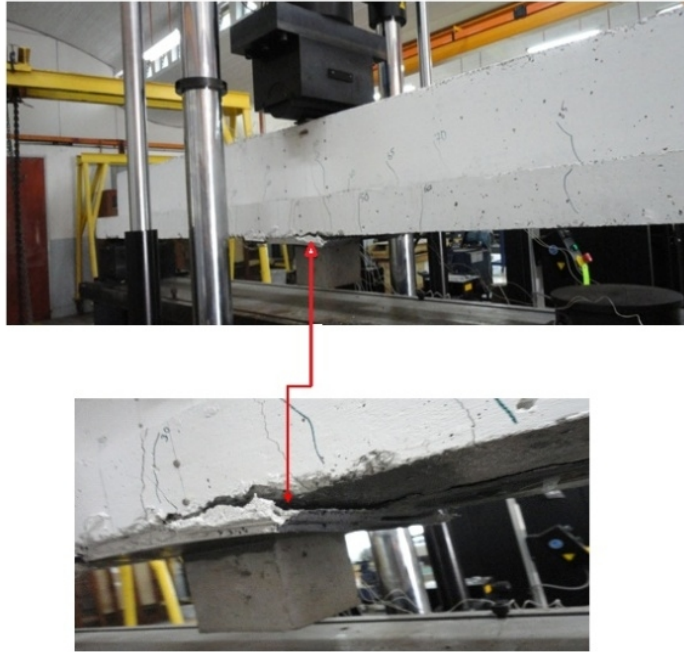
Fig. 10. Failure mode of beam B 2
