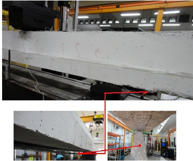
Fig. 8. Failure mode of beam B 0
