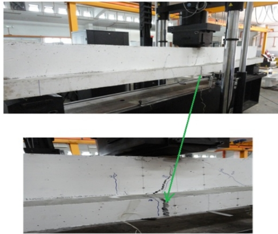
Fig. 9. Failure mode of beam B 1
