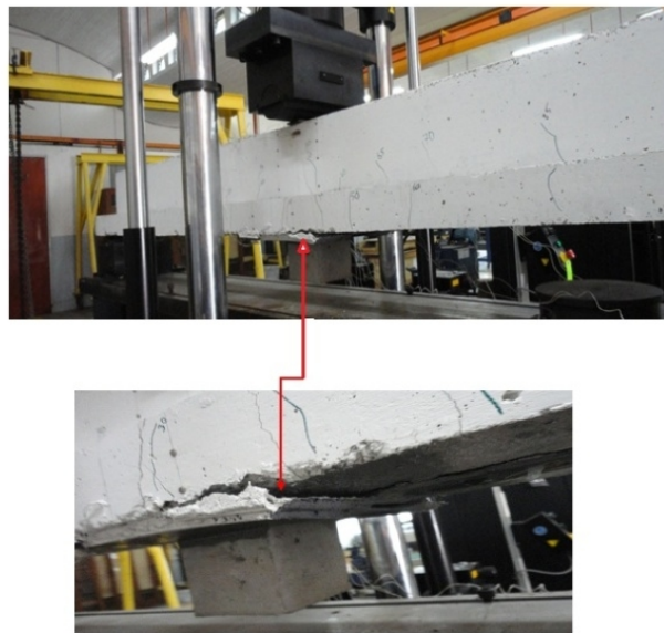
Fig. 11. Failure mode of beam B 3
