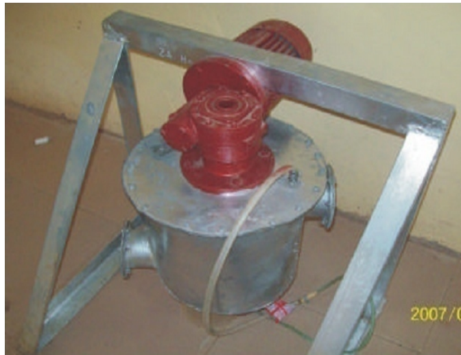
Plate 2.1 A typical laboratory biogas digester (SORCE: Parawira [247])
