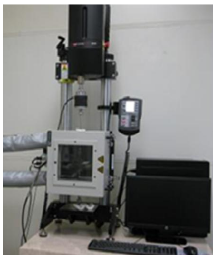
Fig. 1. Instron MicroTester and the corresponding 3-point bend test setup
