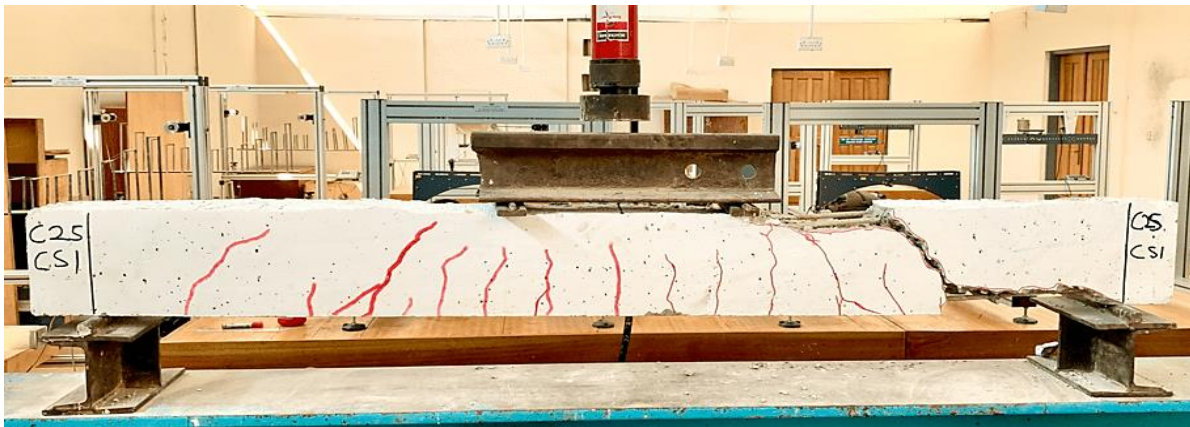
Fig. 6. Beam BG1 failure mode
