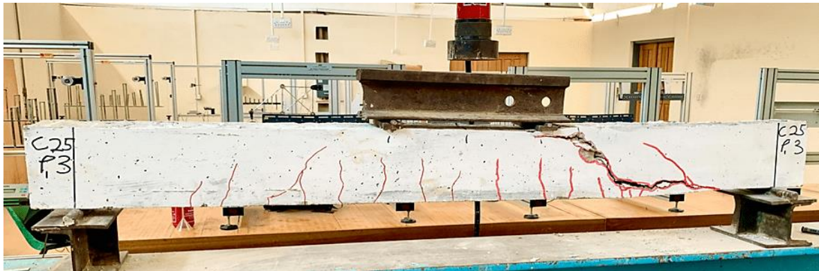
Fig. 11. Beam BG6 failure mode
