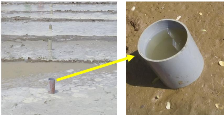
Fig. 2. Infiltration rate measurement
